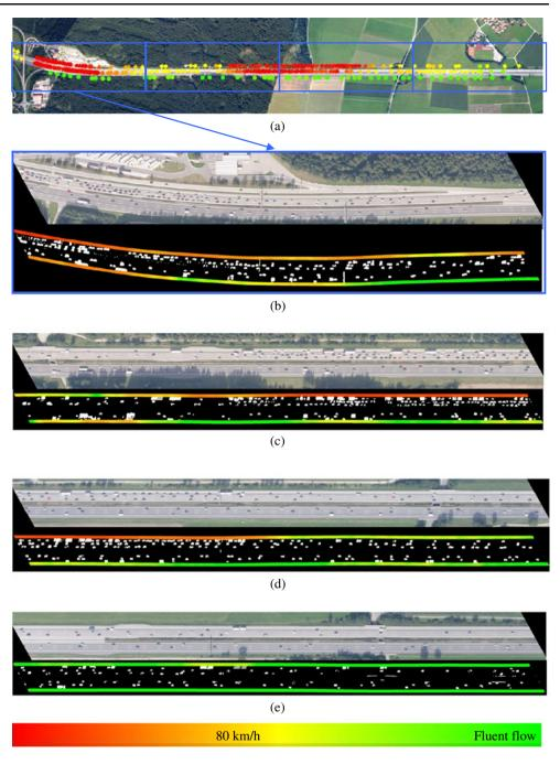
unique definition and it is usually country dependent e.g. see [20]. Having the average vehicle speed for each road segment the congestion detection is a trivial task and can be performed by a simple thresholding. For example, if the congestion is defined for speed up to 50 km/h (for motorways), then the red colored areas in Fig. 5 can be interpreted as congested ones.
