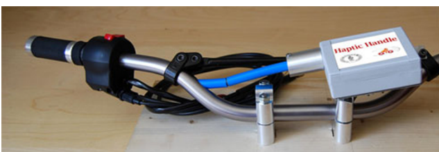
Fig. 7 Haptic Handle ( left ) and electric motor and Control Box ( right )
