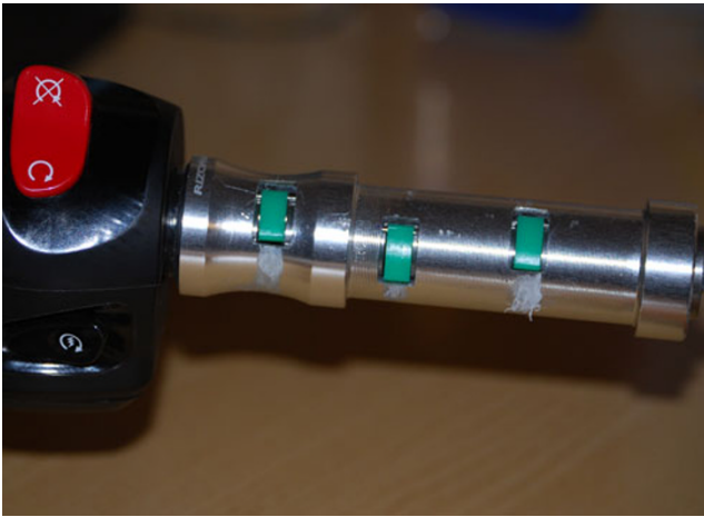
Fig. 6 Moving elements integrated in the haptic handle
