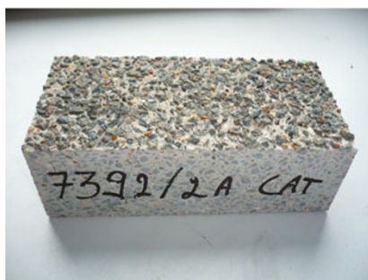
Fig. 14 Effect of different photocatalytic products (1=integrated in cement, 2=TiO 2 powder and 3=TiO 2 suspension) mixed in the mass of the concrete (no curing compound, modified curing procedure)
