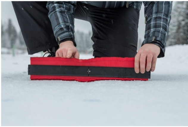
Fig. 1 Measurement of rut depth with a profile gauge
