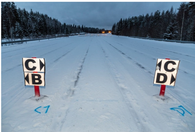
Fig. 5 Compact snow section for constant speed at the end of the test, 50% of vehicles with studded tyres
