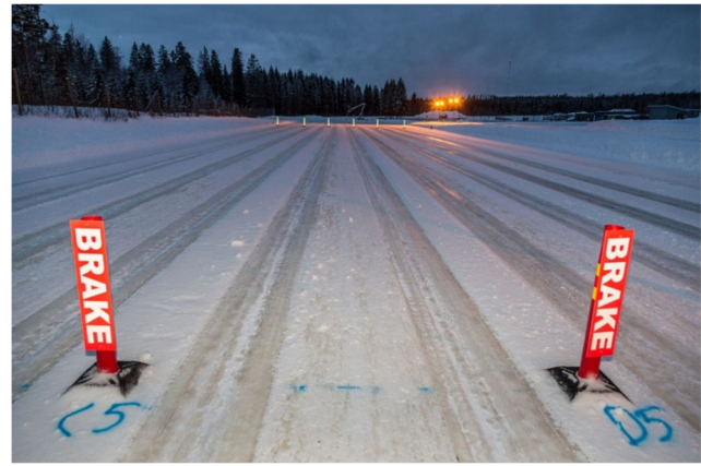
Fig. 3 Icy section for constant speed at the end of the test, 50% of vehicles with studded tyres
