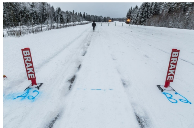
Fig. 4 Compact snow section for braking midway through the test, 100% of vehicles with studded tyres
