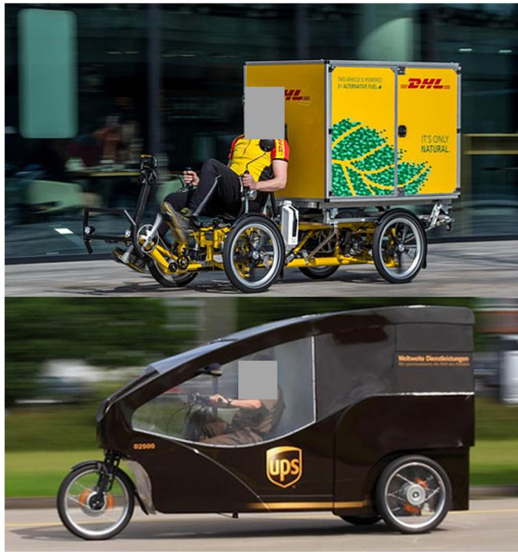
**Fig. 1** Two examples of cargo bicycles. DHL (on the left) [18] and UPS (on the right) [19] are using cargo bicycles in their parcel distribution strategies in Europe and the US
