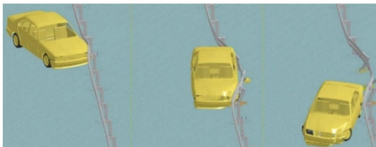
**Fig. 3** Steel barrier, car 1500 kg
