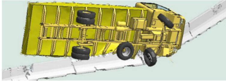
**Fig. 6** Vehicle breaks through a barrier during a simulation test
