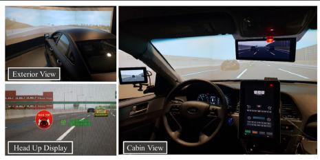
Fig. 1 Internal/external views of the full-scale vehicle simulator
