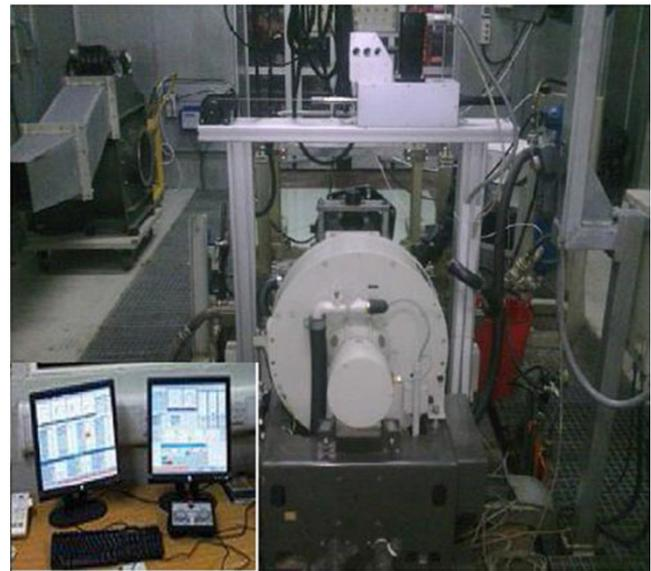
**Fig. 1** Control panel and test engine on dynamometer
